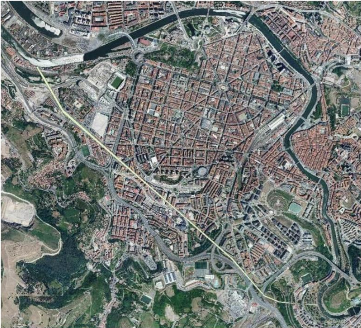
Figure 5. Plan of the tunnel that would deviate river waters from La Peña (upstream, south-east) to Olabeaga (downstream, north-west). Source: ARPSI, Proyecto PGRI 2015-2021.
